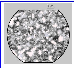
Composite image of ferromagnetic domains in PtMn/[Co/Ni] bilayer, prepared by overlaying several XMCD images. Illustrates switching properties of different FM regions.
